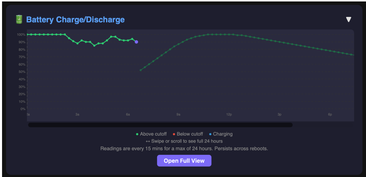
Figure: Battery Charge/Discharge card showing 24-hour battery percentage graph
